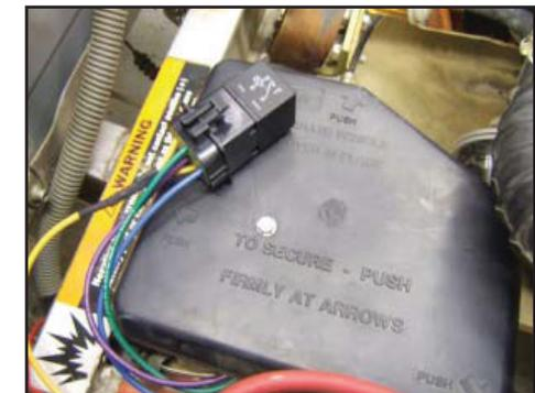
Figure 11 - Relay Mounting Position
