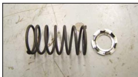
Figure 4 - Spring & Spring Seat Washer
