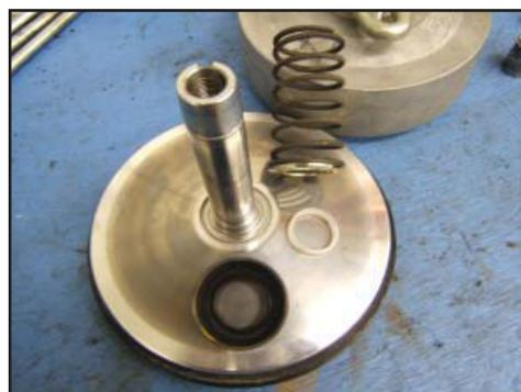
Figure 3 - Spring Removal
