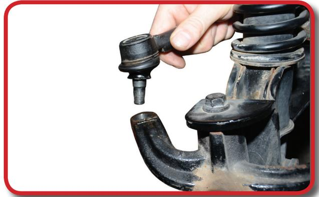
Using a 15mm socket and wrench remove hardware from top of the shock and from the lower control arm. Remove factory suspension assembly from cart. Retain hardware (factory suspension will not be reused).
