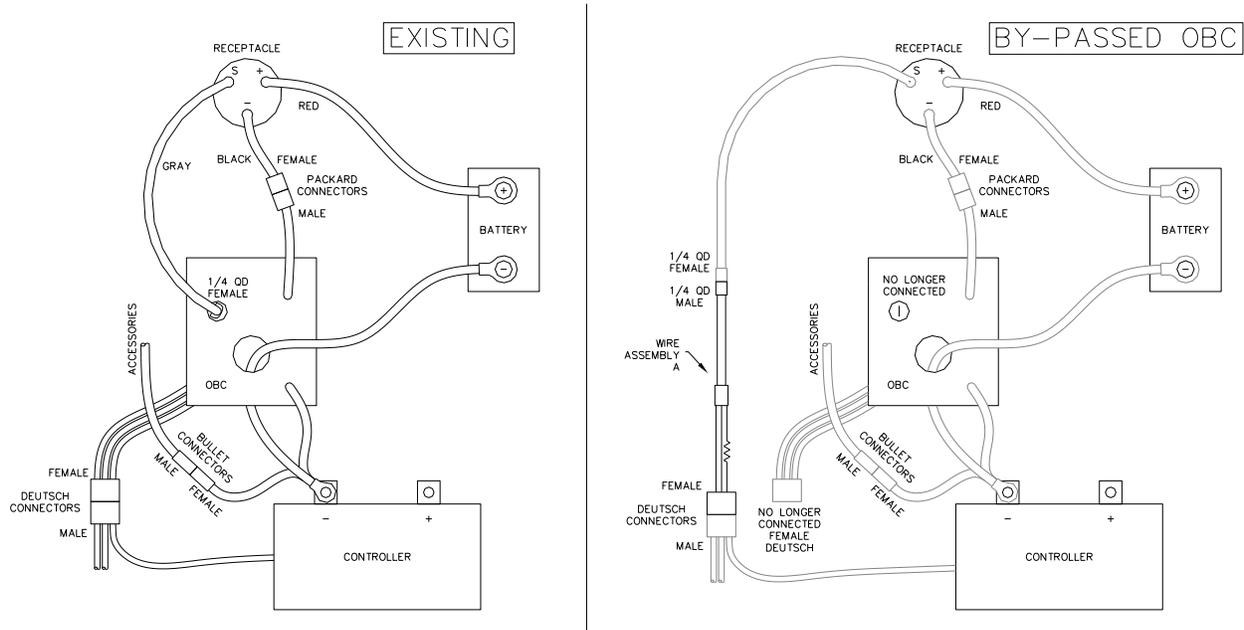
8. **\*For On-Board charger mounting only!** DC cables go directly to battery terminals and the Blue lockout wire from the charger connects directly to the 6 Pin wire assembly A pictured below.
