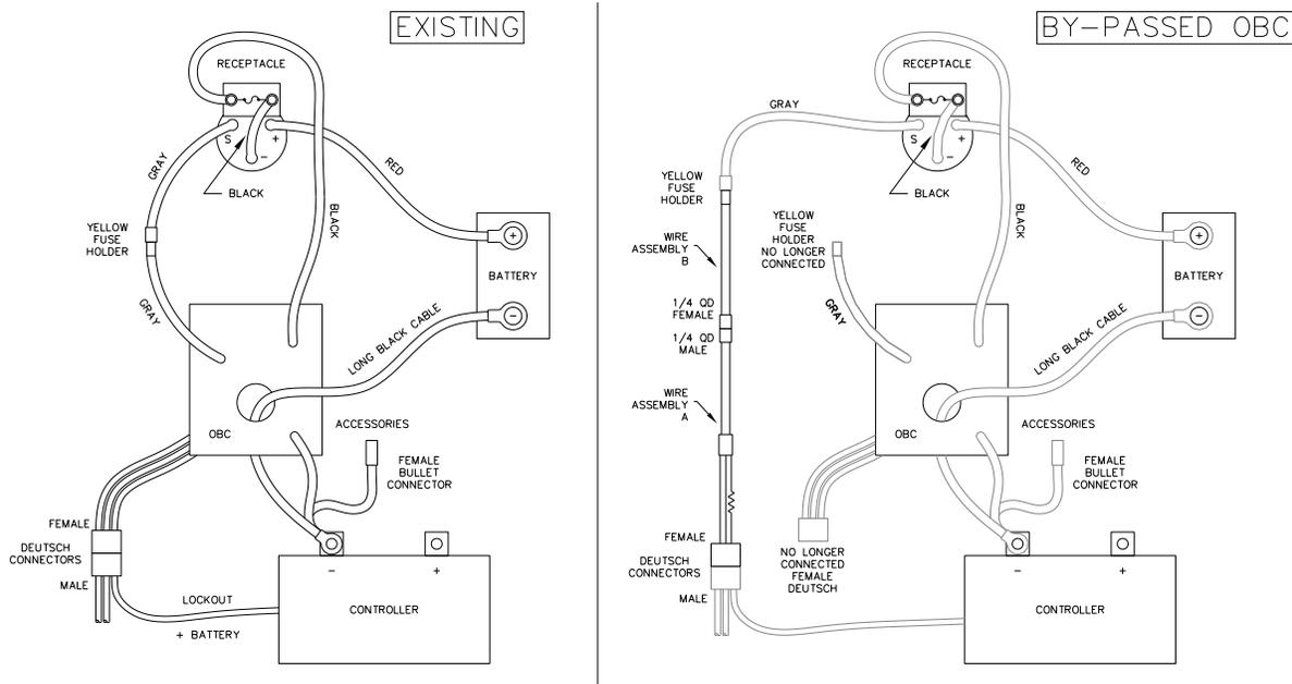
8. **\*For On-Board charger mounting only!** DC cables go directly to battery terminals and the Blue lockout wire from the charger connects directly to the 6 Pin wire assembly A. (Wire assembly B with yellow fuse holder is not used)
