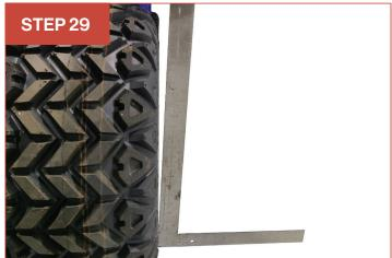
Ensure the steering wheel is straight to begin adjusting the toe of the front tires. The measurement between the center of the tread of the two front tires at the front the should be  $\frac{1}{8}$ "- $\frac{1}{4}$ " **shorter** than the same measurement at the back of the tires.
