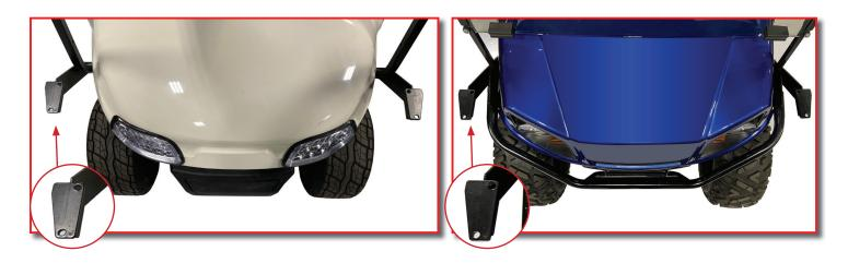
ATTENTION: Ensure that the flat edge of the mounting bracket is facing the inside of the cart as shown.
