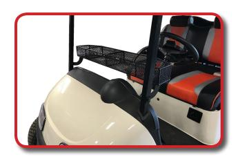
Drill hole through strut with 5/16" Drill Bit and secure mount basket with supplied 8mmx45mm bolts.
