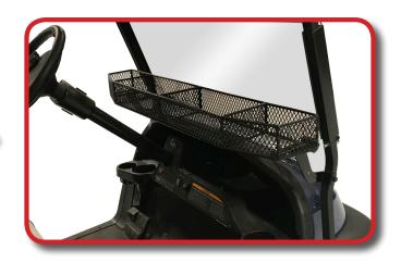
Drill hole through strut and secure using supplied 8mmx40mm bolts, washers and nuts.
