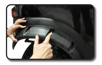
Push the first rivet in to secure fender flare and then insert other rivets.
