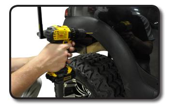
Insert barbed push rivet half-way to secure fender flare. Check other marked holes to ensure proper placement before drilling. Once sure of placement, rotate fender flare out of the way and drill other holes.
