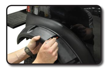
Drill first hole using a 9/32" drill bit. Ensure area behind body work is clear to avoid potential damage to wiring or other bodywork.
