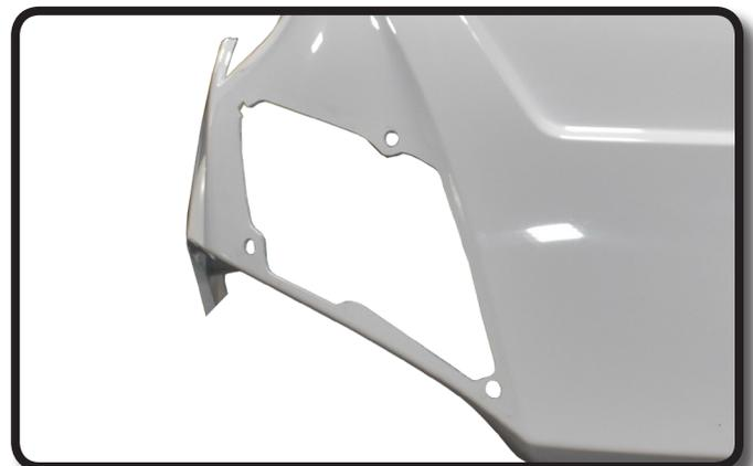
Mount new LED Headlight through the cutout using supplied push nuts.
