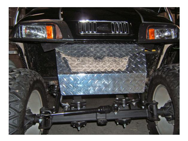
Remove the existing shock shield. You will find in most carts two plastic rivets that will need to be pried out. The upper screws will be removed with either a 3/8" wrench of a 7/16". The new stainless steel hardware will be used for attaching the new cover.
