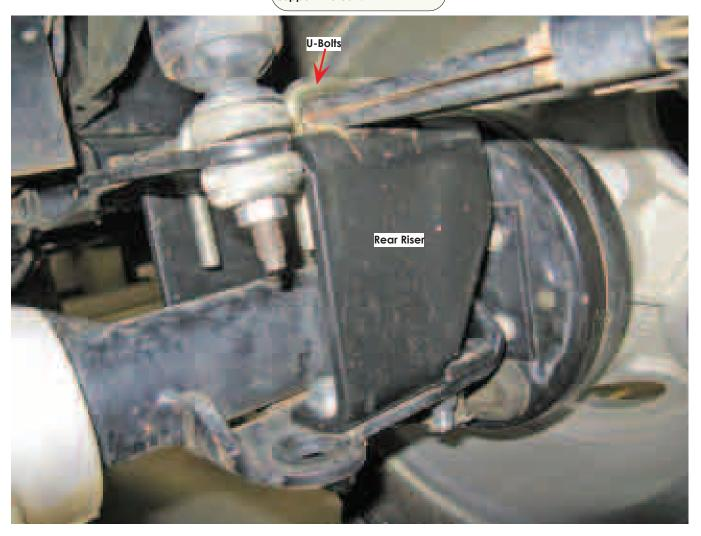
Place a floor jack under the differential housing and apply some pressure. Remove the wheels. Remove the rear springs and lower the drive unit (differential) low enough to accommodate the new riser. With the riser in place set the spring on top and bolt securely to the axle and riser. It will be necessary to remove the lower shock and push it up out of the way and retain the hardware.
