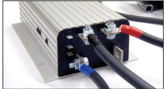
11i. Black Cable Installation on Controller
