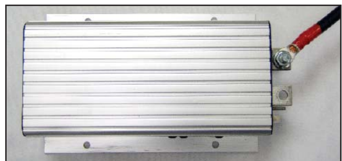
11c. Red Cable Installation on Controller
