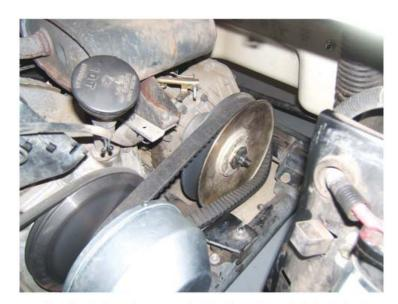
Position the belt as shown and rotate the driven clutch clockwise
