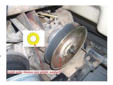
Install the drive belt by placing the belt onto the drive clutch first. Next lay the belt over the top of the driven clutch and rotate the driven clutch clockwise until it is pulled into place.
