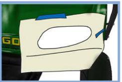
out the inside of the marked area. Test fit the headlight and make any adjustments before removing the tape. Once the light fits, remove tape and sand any rough edges.
