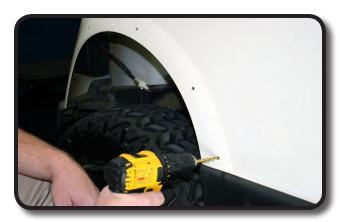
Insert barbed push rivet half-way to secure fender flare. Check other marked holes to ensure proper placement before drilling. Once sure of placement, rotate fender flare out of the way and drill other holes.
