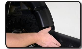
Push the first rivet in to secure fender flare and then insert other rivets.
