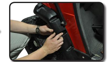
Push the first rivet in to secure fender flare and then insert other rivets.
