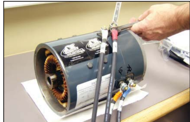
11d,f,h & i. Motor Cable Installation
