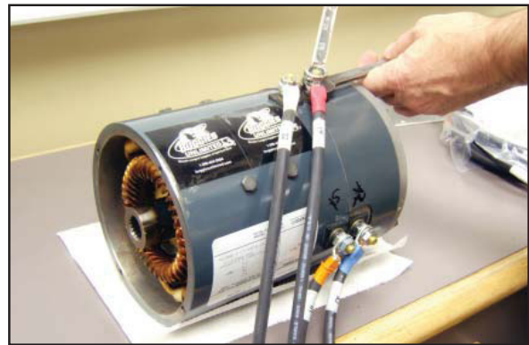
11d,f,h & i. Motor Cable Installation
