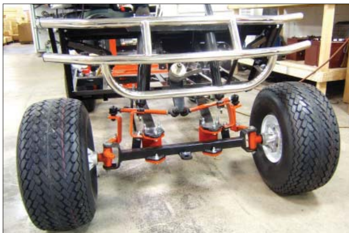
Brush Guard Installed
