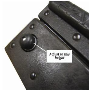
Drill holes in the pedal as per above. Yamaha will look different but uses the same fitment. Make sure drilling does not hit any moving parts.
