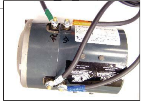
16. Orange Cable Installation
