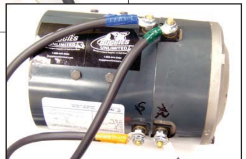
13g. Orange Cable Installation
