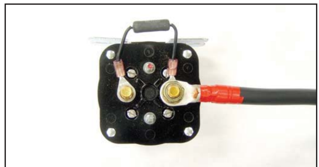
13b. Red Cable on Solenoid
