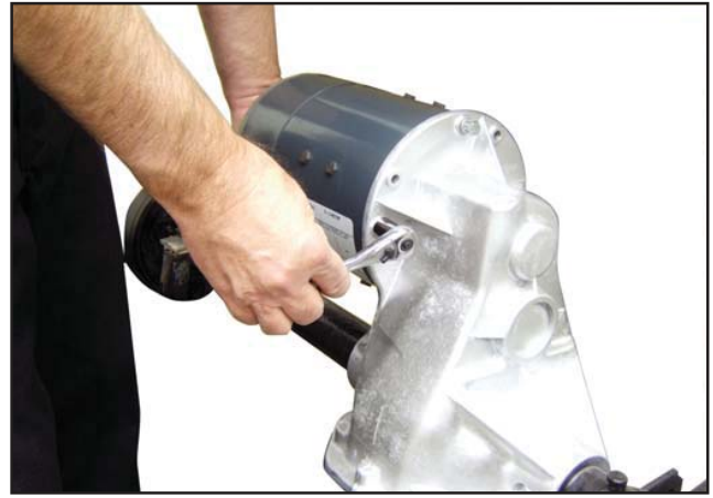
10a. Motor Installation
