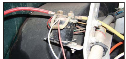
6d. Solenoid Mounting 2
