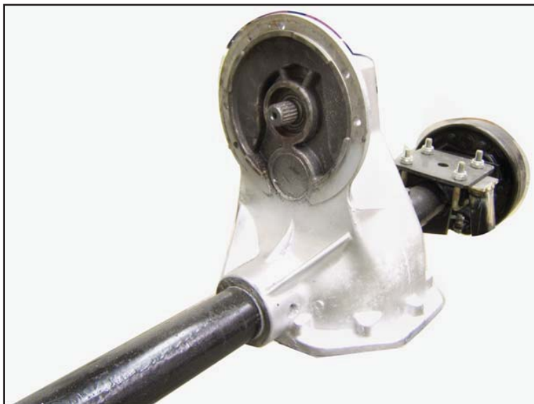
9. Clean the Motor Mount Area
