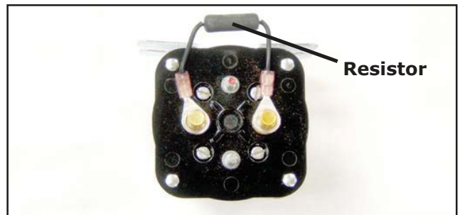
13a. Resistor Installation
