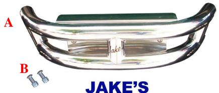
Hardware: 5/16 x 1 Stainless Steel Button Heads w/ Locknuts-2 ea.
