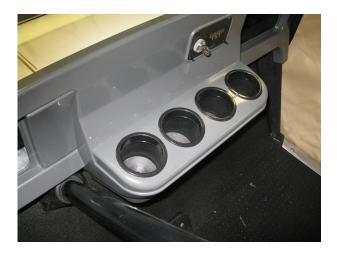
Place the new cover over existing dash area. You will need to use great force to push the cup holders into place. Do not hit with hammers! Hard pushing and manipulation will work the cover on!
