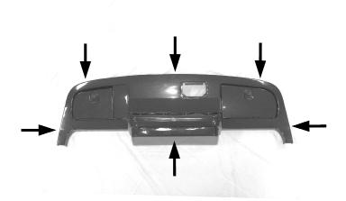
Drill 1/8" holes in the area's marked and install screws.
