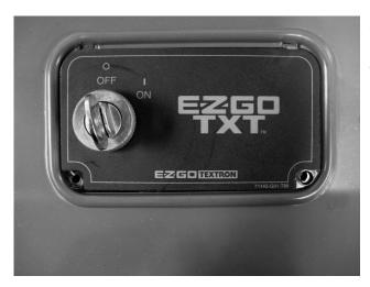
On the key switch plate remove the center push pins on black rivets. Park in an area they can fall to so you can find them. Place key switch plate on new dash and install plastic rivets and center push pins.
